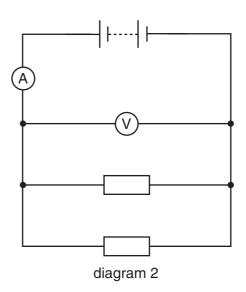
What are the ammeter and voltmeter readings in the circuit shown in diagram 2?
