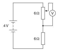
What are the minimum and maximum readings that can be obtained on the voltmeter when the potential divider is adjusted?
