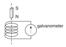
The magnet moves through the coil and, as it falls away from the coil, the galvanometer pointer
